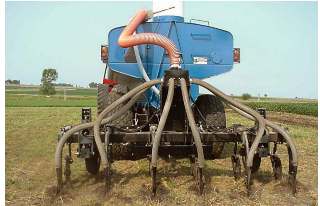
Tool bar with hydraulic injectors - undersurface spreading -
